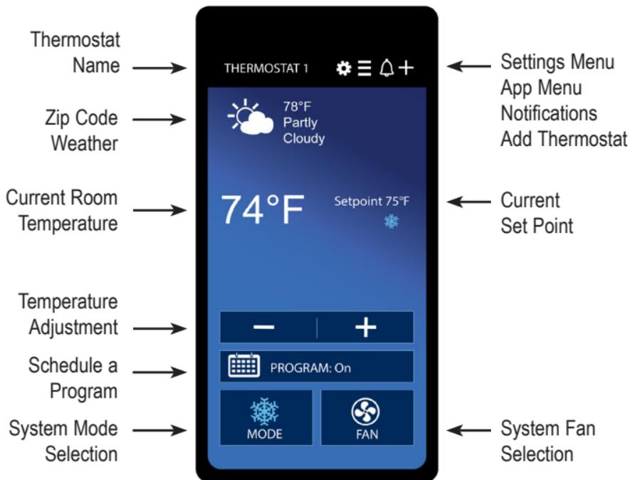
**Temperature Adjustment** - The plus and minus buttons are used to adjust the current setpoint. If set to programmable operation, adjustment will create an **OVERRIDE**. The override can be cancelled by pressing the Cancel Override button.
