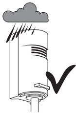
**MUST BE MOUNTED CABLE INLET FACING DOWN**
