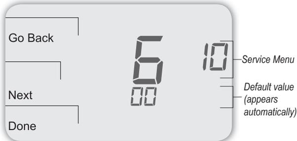
3. In Service Menu 610, press **▲** / **▼** to select option "01," Heat Stage 1 (see Fig. 12). **Note:** If 01 is selected, the thermostat will activate the associated output for up to 10 minutes. The user should observe that the fan output (with heat) turns on. The user may also test more stages of heat according to what is available for the system type.
